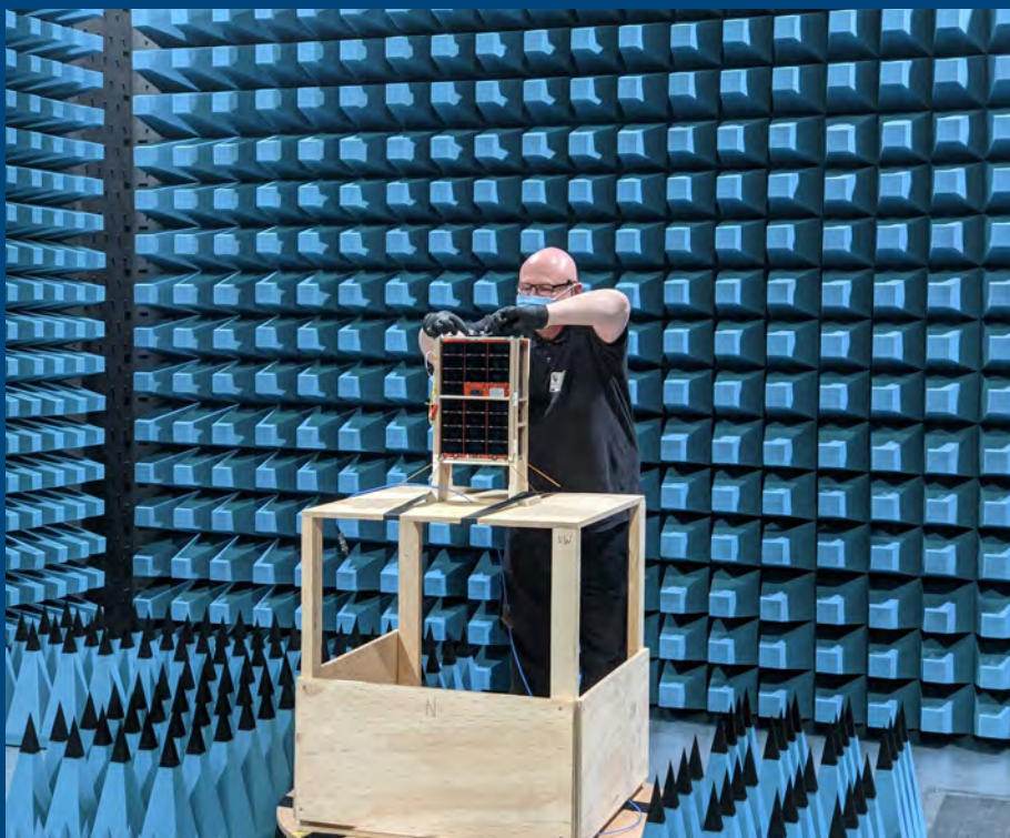
↑ A DSTG Engineer attaches a radio frequency cable to the engineering model spacecraft during anechoic chamber testing of the Buccaneer Main Mission nanosatellite, which was launched from the United States into low earth orbit in April 2025.
