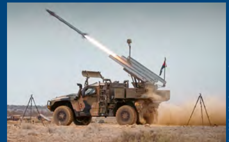
↑ An Army Hawk high-mobility launcher from 16th Regiment fires an AIM-9X Sidewinder missile at the Woomera test range in South Australia.
